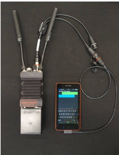
PriveTAK handheld terminal with 4W Silvus Streamcaster 4240 node
