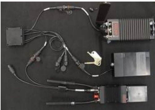
Used equipments to establish an encrypted tunnel over LTE network from Battalion HQ to XXLSEC office
