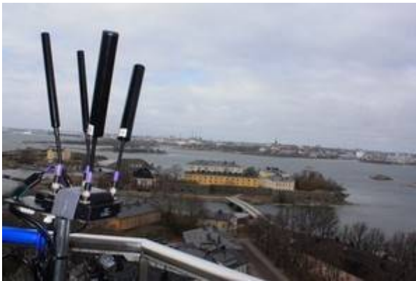
Silvus Streamcaster 4480 8 W MESH node at Company HQ facing towards Battalion HQ.
