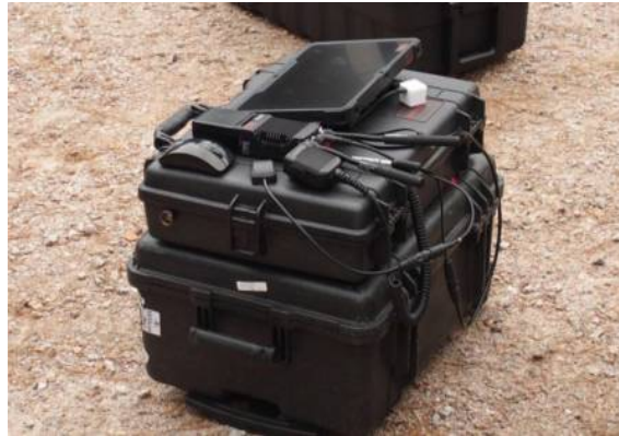
Platoon leader Silvus Streamcaster 4240 4 W MESH node and Tactical Server at Special Mission area #1
