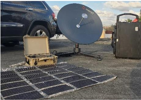
When cellular and terrestrial connectivity is lost due to infrastructure damage, prolonged power outages, or even cyber-attacks, satellite can often be the only form of connectivity available. With the right service provider, it provides a robust, reliable form of IP connectivity for internet, voice, and data services.
