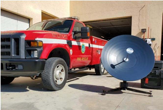
**EOC Site** - A 7 Mbps satellite IP data link was deployed at the Islamorada Emergency Operations Center (EOC) in the center of the main island, along with a Silvus StreamCaster 4400 IP MIMO Radio and a high-gain 19dBi panel antenna. The IP radio was connected to a Cisco Meraki router, which was connected to the iDirect satellite modem.
