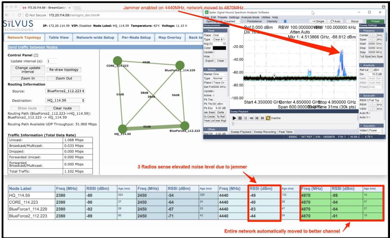
Figure 7: Silvus network has switched over to 4870 MHz channel after interference was introduced in the 4400 MHz channel.
