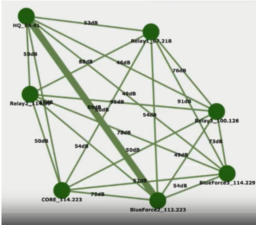
Figure 8: Start of tour in WTC Back of the House. All radios in direct contact with the HQ laptop. Green links have > 20 dB SNR.
