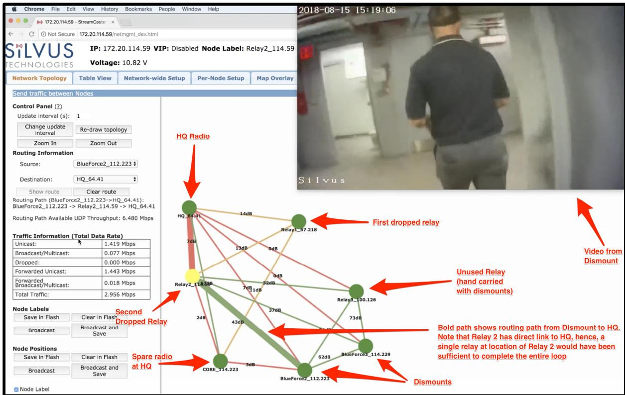
Figure 10: Near the end of the second tour. Relay 2 is providing a strong, direct link between HQ and all of the dismantled radios. Relay 1 was not necessary and is not being used. Fat lines indicate links being used.
