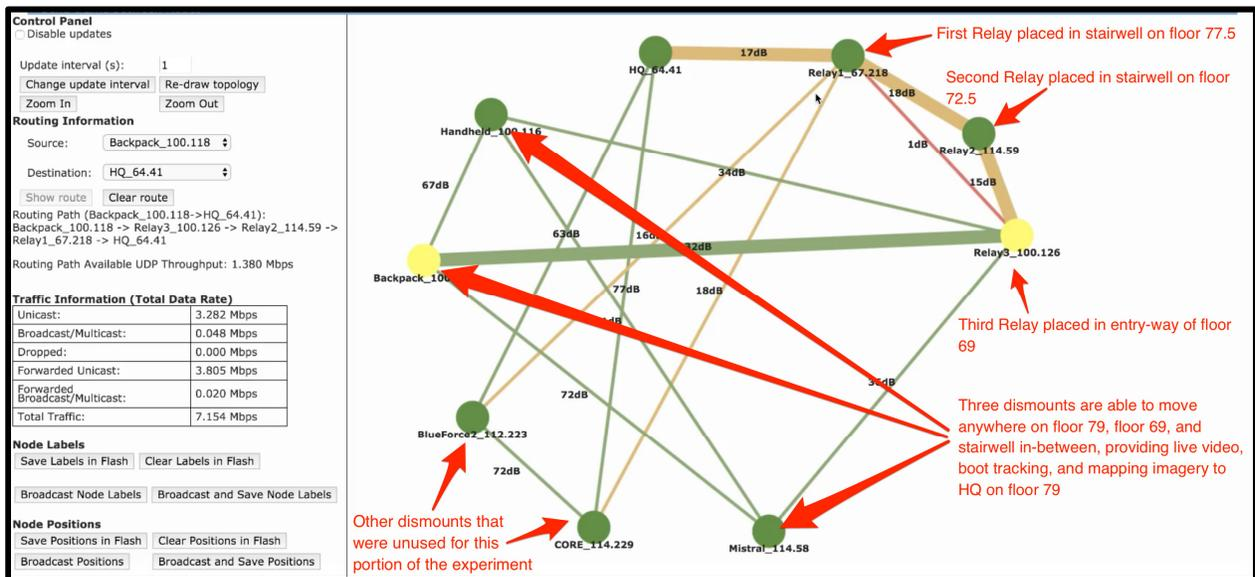
Figure 12: Radios placed in the stairwell near the 77<sup>th</sup>, 72<sup>nd</sup>, and 69<sup>th</sup> floors provided the capability to transmit video, voice and data from anywhere on the 69<sup>th</sup> to the HQ laptop on the 79<sup>th</sup> floor.
