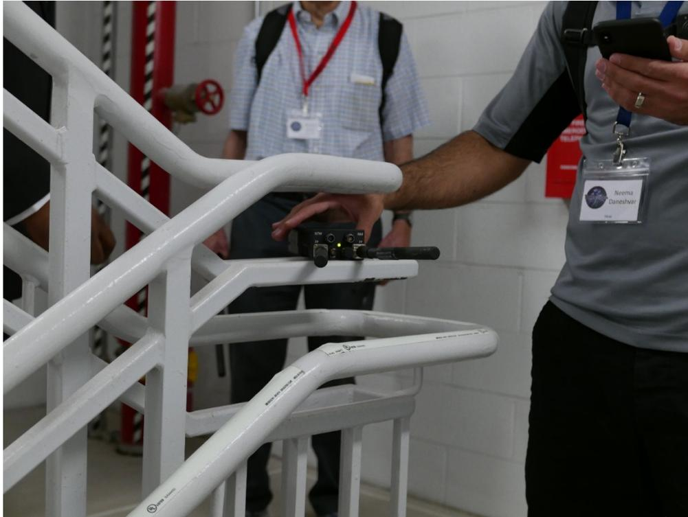
Figure 11: Silvus mesh radio placed in the stairway between the 79<sup>th</sup> and 69<sup>th</sup> floors of NYC Skyscraper.
