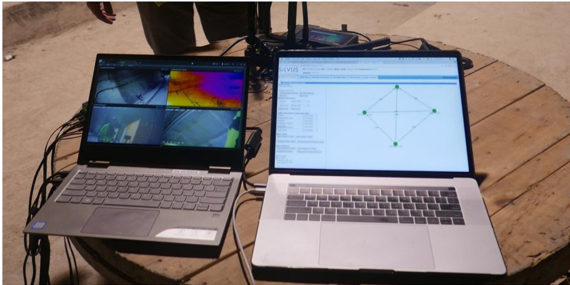
Figure 4: Silvus laptops running StreamScope in the ESA tunnel. The laptop on the right shows the nodes (radios) comprising the network, including the SNR of all inter-node links. The left laptop displays video feeds from cameras connected to radios.
