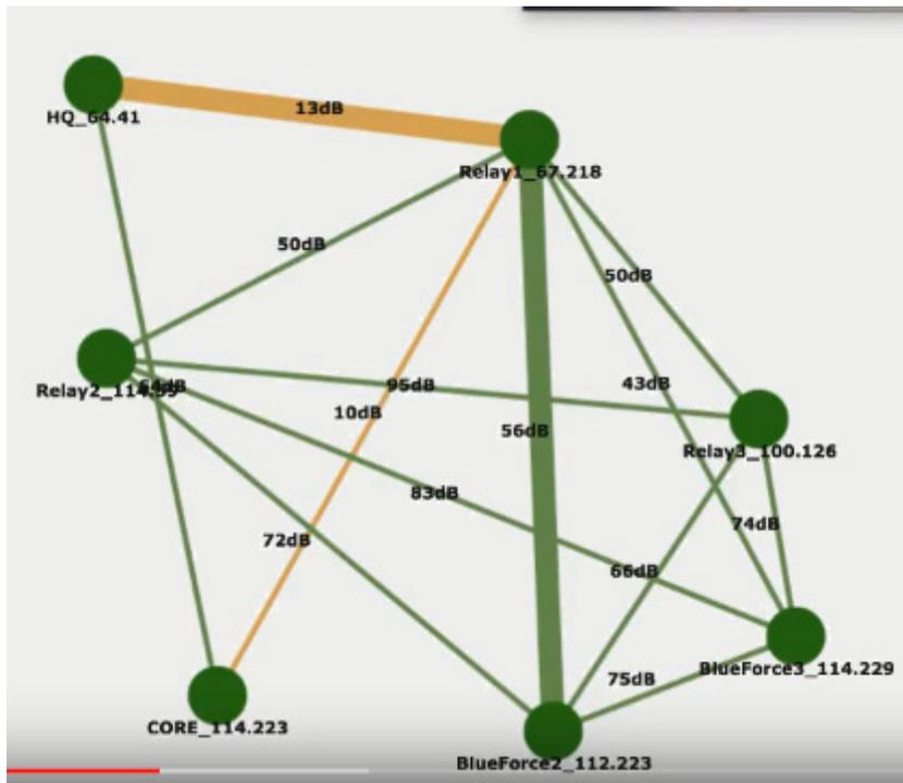
Figure 9: Shortly into the tour at WTC Back of the House. Relay 1 has been deployed along the route and it providing communications with all other radios. Only Relay 1 has direct contact with the Base Station. The CORE radio was left at HQ.
