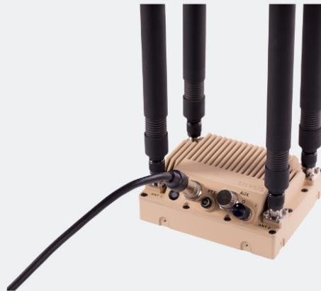
Figure 2: Silvus Technologies StreamCaster 4400 Tactical MIMO radio designed for fixed sites (from company website).
