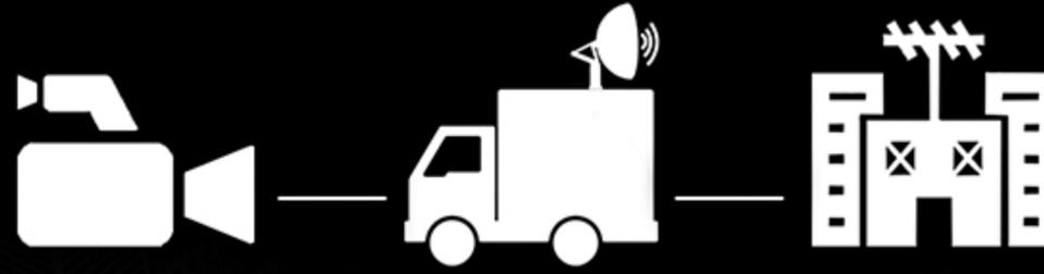
Traditional Electronic Newsgathering (ENG) involves transmitting live video from camera, to an ENG truck, and on to the news station over a series of independent COFDM video links. While this approach generally provides reliable connectivity, it has several drawbacks, namely:
