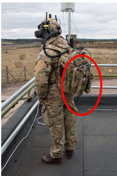
Figure 2. The mobile unit with StreamCaster radio circled
