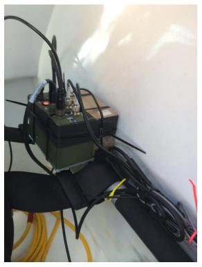
It is notable that the antennas had to be installed inside of the cockpit. The ability to deploy multiple antennas (MIMO) allowed sufficient flexibility in choosing antenna locations within the cockpit, that in the aggregate, good RF coverage could still be achieved without any antennas mounted on the outside of the boat.
