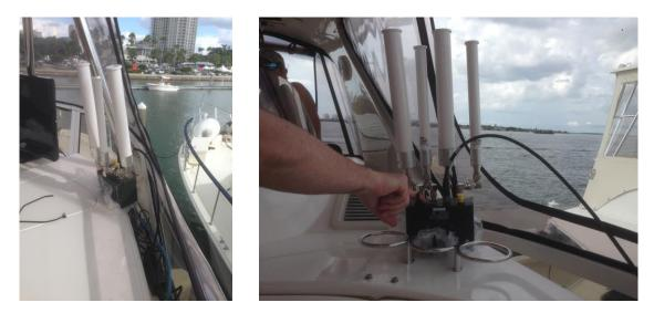
It is worth noting that for ease of install, the radios were mounted inside the cabin of the boat, not above the cabin where the permanently installed comms antennas and radar were positioned. However, full 360 degree coverage was still assured by deploying two radios (one of each side of the cabin).
