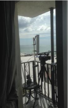
The antennas were positioned on the balcony with one pointed up towards the north end of the course and the far turn boat, and the other antenna pointed towards the south side of the course and the finish-line boat. Both antennas had a slight mechanical down-tilt.
