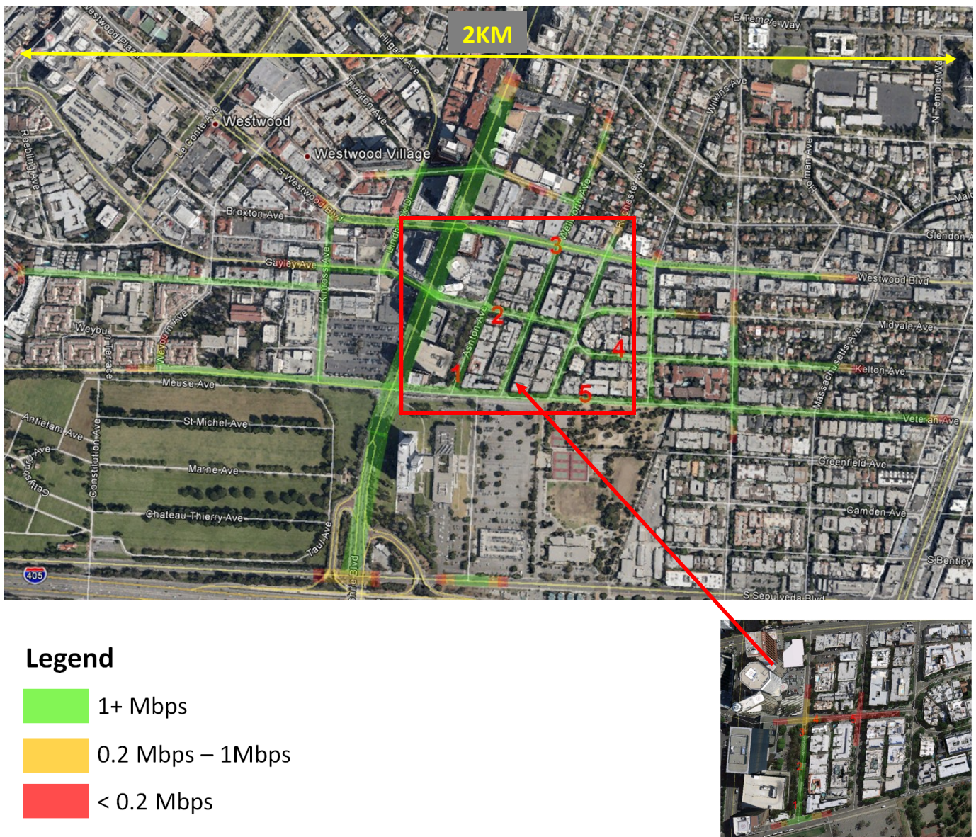
Figure 2. StreamCaster™ 3500 Mesh Coverage with 1 Watt Nominal Power (Above), compared with 802.11n 50mW coverage (Below)
