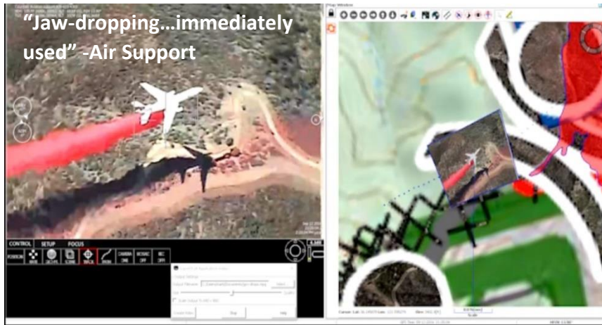
Hands-off retardant drop tracking with live mapping
