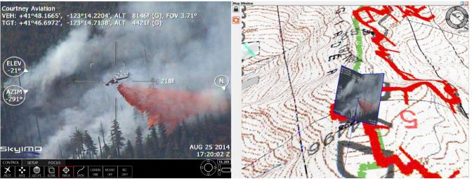
Video of a Sky Crane dropping retardant on the Happy Camp Complex wildfire transmitted live to the ground Incident Command. Live microwave linked 28 miles to SkyIMD's IR/EO from the base station. Live control occurred in the field, and was transferred through the internet to Incident Command, where the Planning Section Chief could operate the superzoom gimbal.
