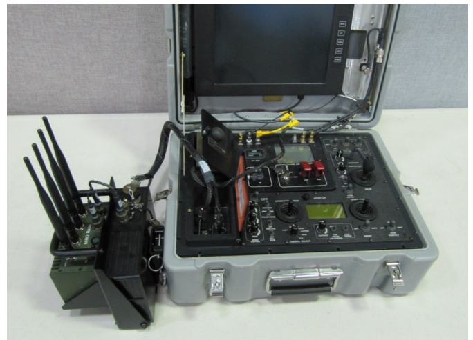
Figure 2. Silvus SC3500 integrated into TALON OCU
