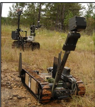
Figure 1. Silvus SC3500 integrated into FasTac & TALON, note the Silvus radio on the ground with the soldiers
