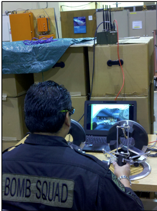
Figure 1. Silvus SC3500 MIMO Radio in background used by Bomb Squad tech operating Taurus on an Andros robot
